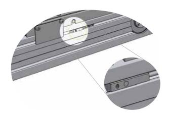
These inductive switches are the most compact version of switches. These switches are flush with the surface profile and therefore you will have almost no interfering edge.
