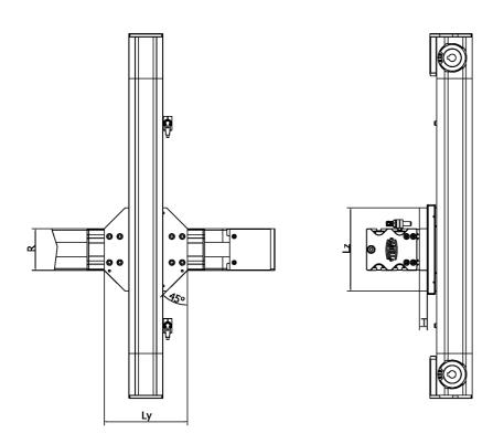
Centre of actuator = centre of carriage plate Adjustment using cylinder pins or stop angle
