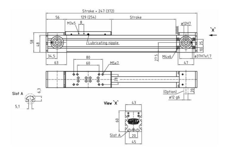
Stroke calculation: using distance and safety overrun Values in brackets for long carriage Motor connection see chapter Drive adaption
