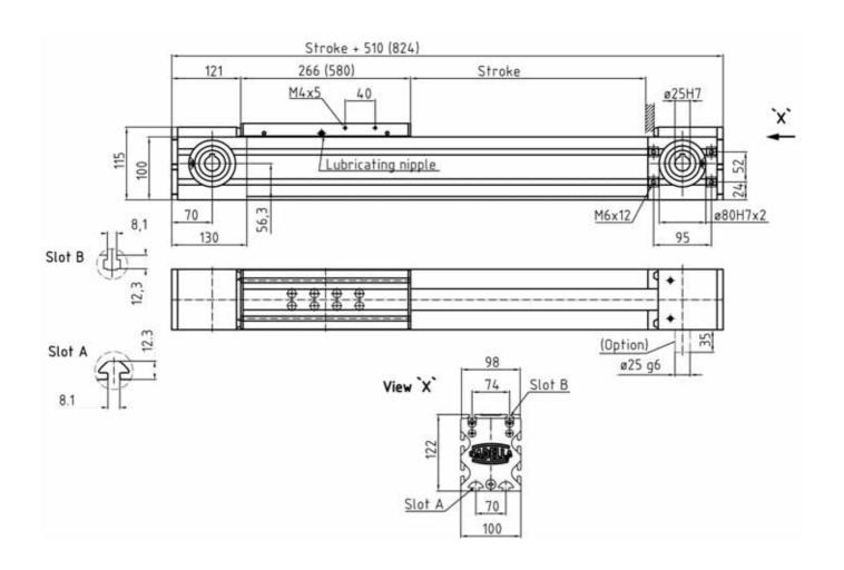
Stroke calculation: using distance and safty overrun Values in brackets for long carriage Motor connection see chapter Drive adaption
