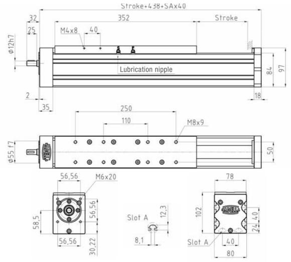
Stroke calculation: effective stroke + safety overrun SA = number of spindle support sets For motor connection see chapter drive adaption Lubrication: S = ball screw; F = rail guide
