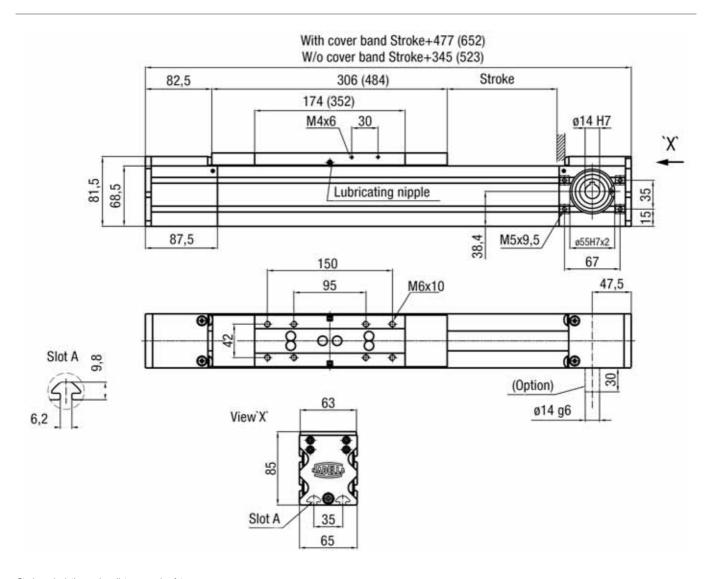
Stroke calculation: using distance and safety overrun Values in brackets for long carriage Motor connection see chapter Drive adaption
